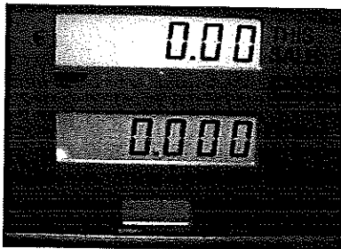
Fig1. Wayne dial face with Fault LED Note: On Tokheim Dial Face LED is separate at the left hand end of the litres display
